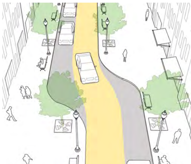
Chicanes are offset curb extensions that reduce speeds and increase public space along a corridor. Source: NACTO
